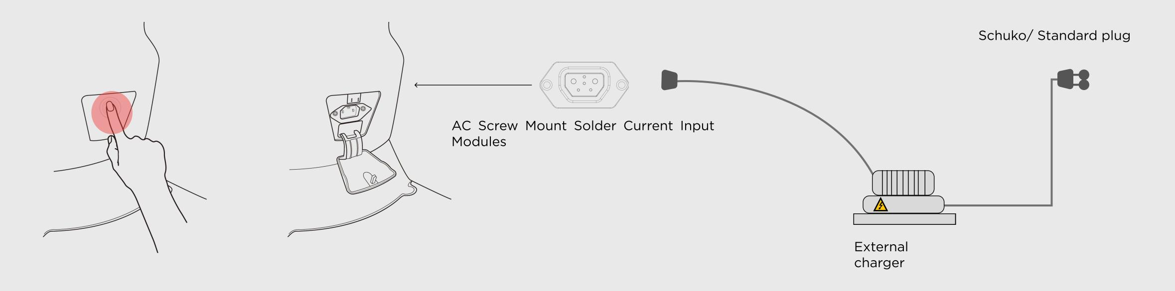
Gently press the top part of the cover, where the connector is located, to access the charging socket. Take the charger, plug it in, a light will go on when it is fully charged
