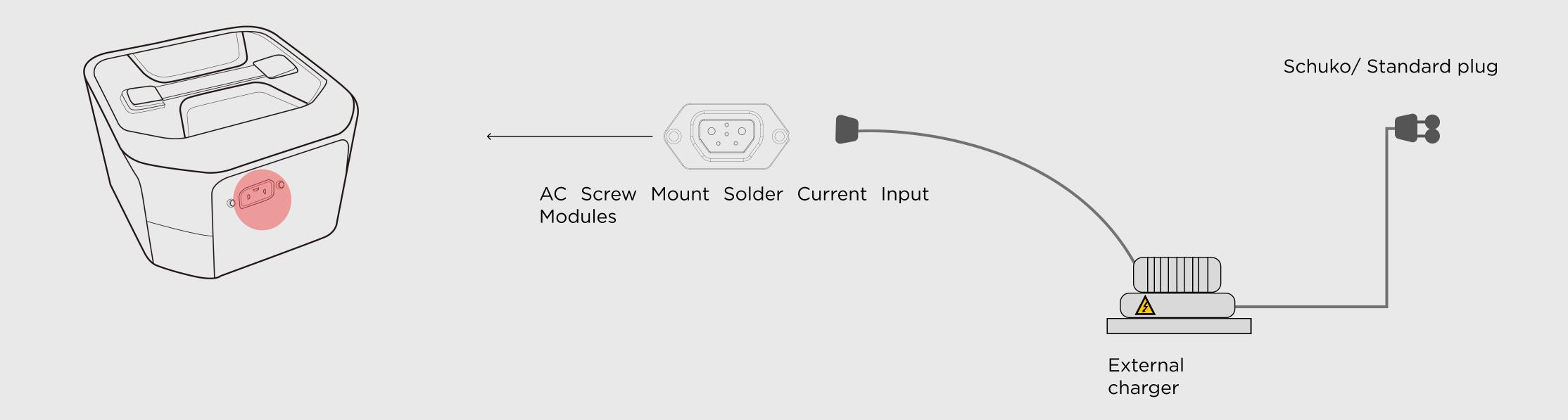
First open the top box, then unlock it using the key to access the battery compartment. The lithium battery can be removed to charge it in the most convenient place. Please, use the original NEXT charger for lithium batteries, and there is a light on the charger that shows the charging status
